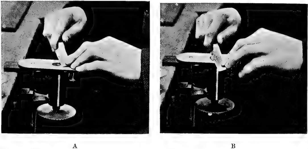
FIG. 14.—Photographs of the operator in the act of cutting sections. A, showing the point of the knife in contact with the specimen. B, showing the position of knife at completion of cut, with the section resting on the blade and the paraffin curled over in front of it. The movement of the cut is a sliding one, its traverse being from right to left, the full length of the blade having been used in the operation.
